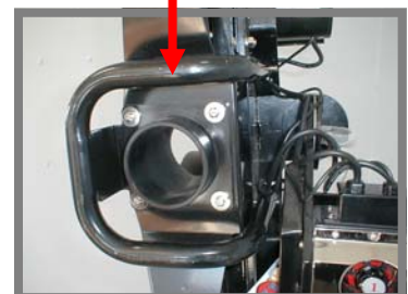
Feed Chute Installed
